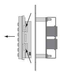
Once the keypad cover has been removed, pull a button off and replace it with one of the optional buttons.
