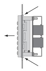
2. Using a small flat blade screwdriver, release the four tabs on the sides of the module, releasing the keypad cover.
