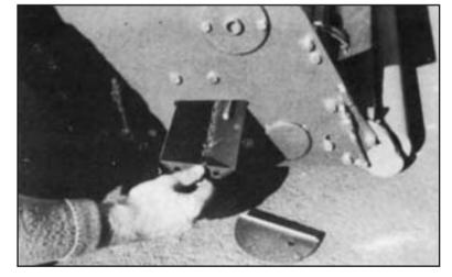
A grass trough is incorporated that can be adjusted closely to the rear drum so that grass and dirt build-up is scraped from the drum and caught in the trough.
