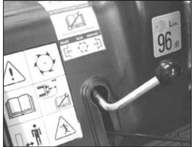
Figure 4. Cutter drive clutch lever.
