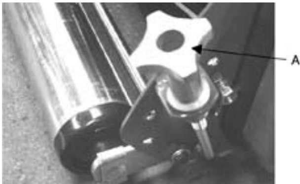
Figure 9. Cutting height adjustment
