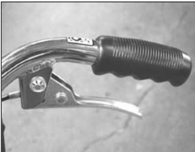
Figure 3. Drive clutch lever.
