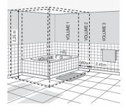
■ The safety rules define three volumes in a bathroom (see diagram 5). this unit must only be installed in volume 3 of the room so that the selector button (A) cannot be touched by anyone using the bath or the shower.
