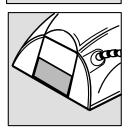
To fold handle , press handle release button on the rear of the iron.
