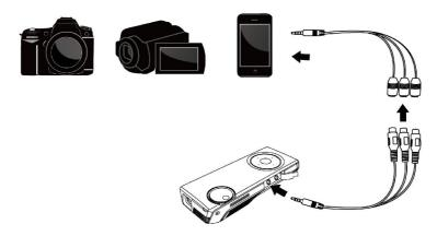
Some video devices do not have the standard audio and video connections and may require an AV cable specified by the vendor. The AV cable allows you to connect your video device to your TV monitor or your projector. Also may be purchased from the video device vendor. When you have the AV cable, use the cable adapter to connect the video device cable and The RMP-8200 CINEMA ON-THE-GO cable.
