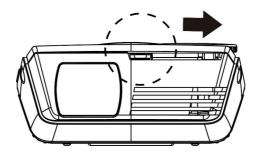
Switch on the power button. From "O" side to "I".
