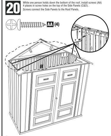
Caution: When installing screws do not overtighten.
