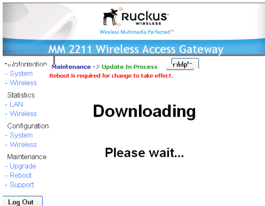
Figure 19—Upgrading Software in Process
