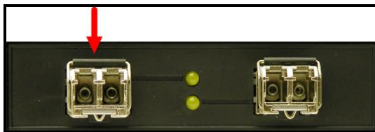
Figure 28: SFP Bail Latch location
