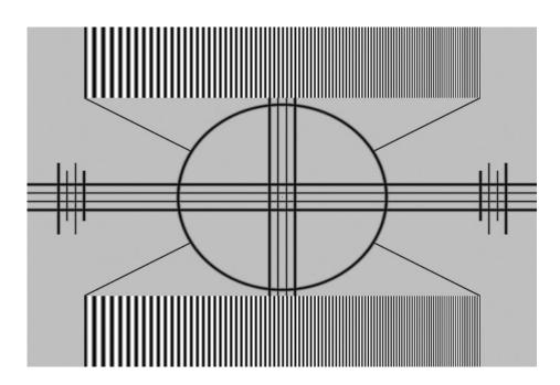
Figure 4-5. Typical Test Pattern for Adjusting Sharpness
