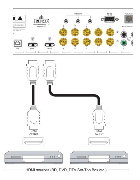
Figure 3-6. HDMI Source Connections
