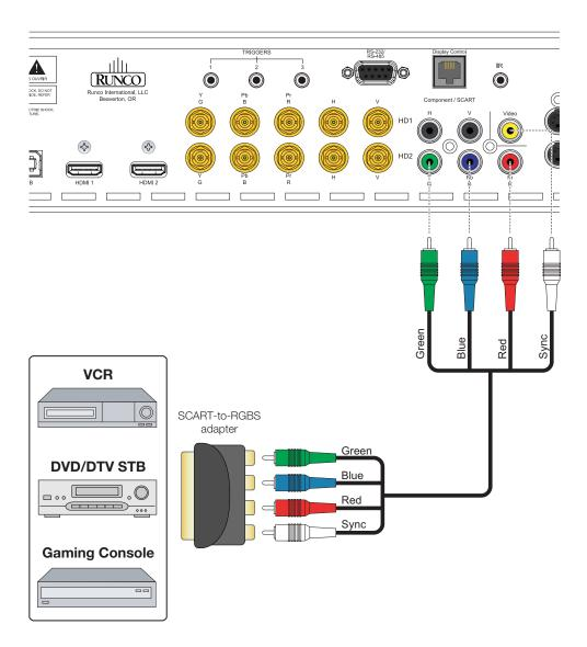
Figure 3-9. SCART RGBS Source Connections
