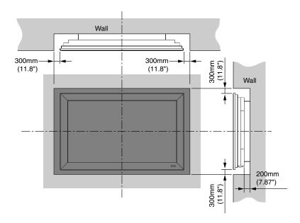
Figure 3-3. Ventilation Requirements for Enclosure Mounting (XP-103DHD)
