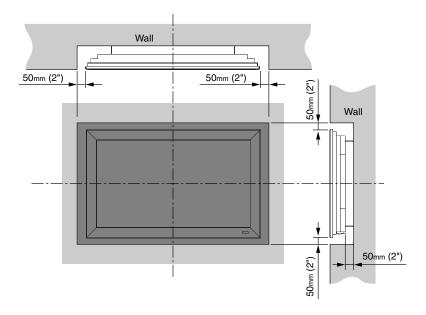
Figure 3-2. Ventilation Requirements for Enclosure Mounting (XP-50DHD, XP-0PAL50DHD, XP-65DHD and XP-0PAL65DHD)
