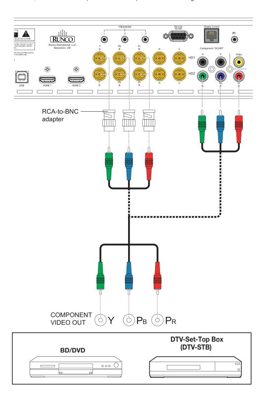
Figure 3-7. Component Video Source Connections
