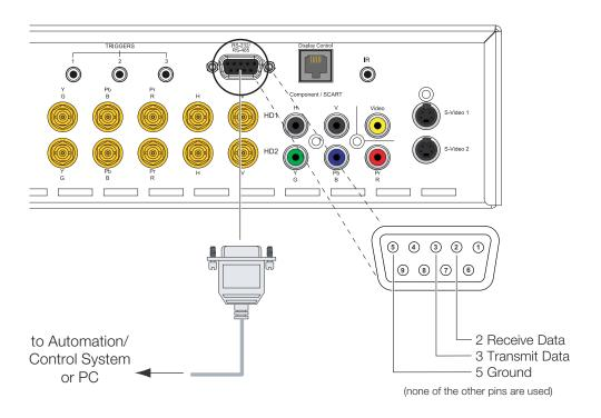
Figure 3-11. RS-232 Control System Connection
