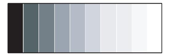
Figure 4-3. Typical Gray Bar Pattern for Adjusting Contrast
