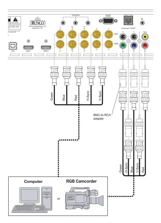
Figure 3-8. RGBHV Source Connections
