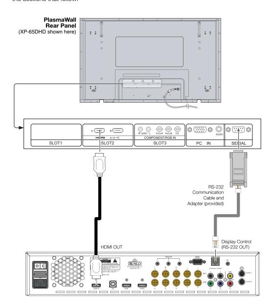
Figure 3-4. Connecting the PlasmaWall to the DHD Controller
