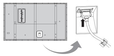
Figure 3-14. AC Power Connection
