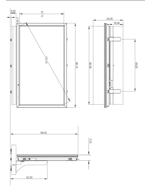
Figure 7-3. PlasmaWall Model XP-103DHD Dimensions (with Floor Stand)
