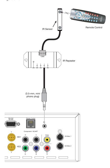
Figure 3-13. External IR Receiver Connection
