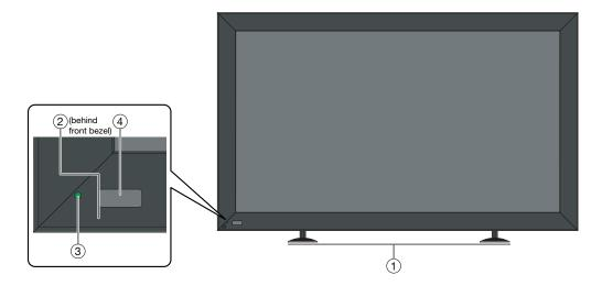
Figure 2-1. PlasmaWall XP-50DHD and XP-OPAL50DHD Front-Panel Controls and Indicators
