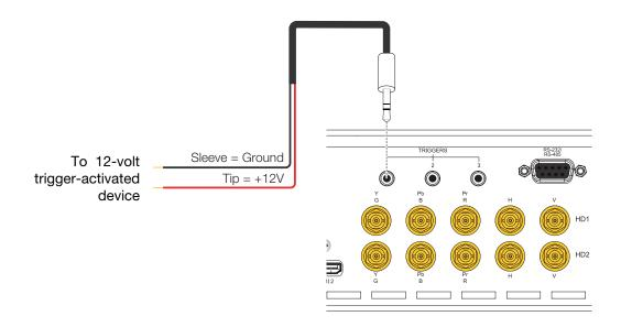
Figure 3-12. Connecting 12-volt Trigger Outputs
