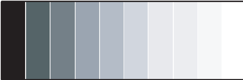
Figure 4-2. Typical Gray Bar Pattern for Adjusting Picture Level (Contrast)
