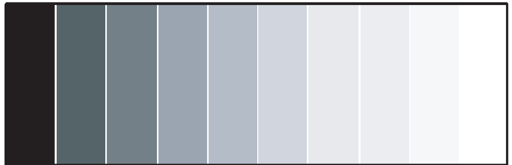
Figure 4-3. Typical Gray Bar Pattern for Adjusting Contrast
