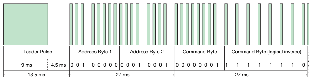
Figure 6-1. NEC Protocol Message Format
