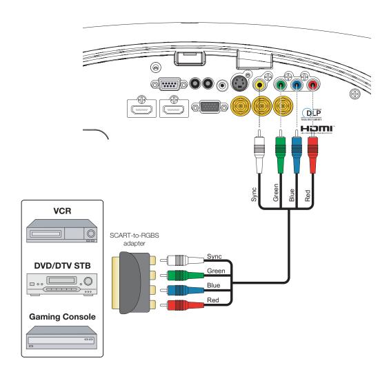
Figure 3-10. SCART Source Connections
