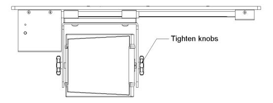
Figure 3-16. Attaching the Anamorphic Lens to the Lens Mount
