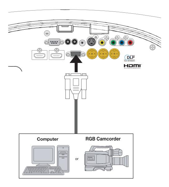
Figure 3-9. RGBHV Connections
