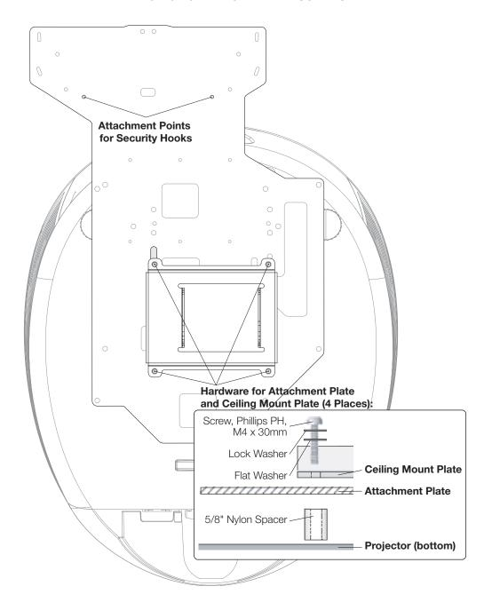
**Installing the Anamorphic Lens Transport Assembly:** After installing the Transport Assembly Attachment Plate and Ceiling Mount Plate, proceed as follows to install the Anamorphic Lens Transport Assembly.
