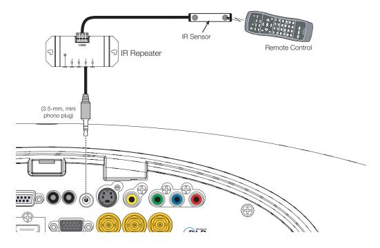
Figure 3-15. External IR Receiver Connection
