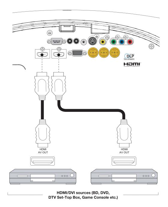
Figure 3-8. HDMI/DVI Source Connections
