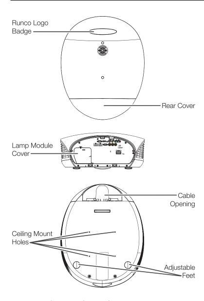
Figure 2-2. LS-10i Rear/Bottom/Top View
