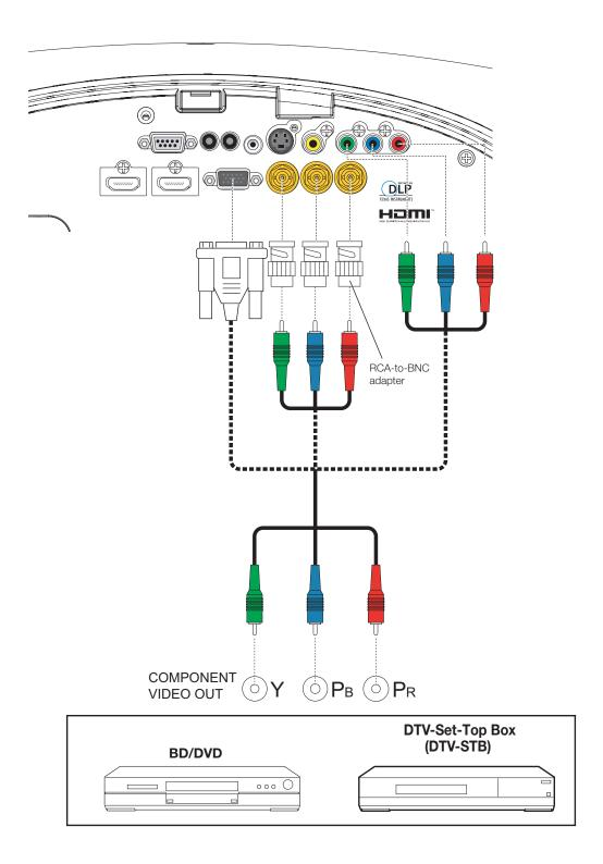
Figure 3-11. Component Video Connections
