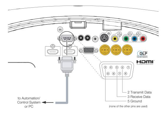
Figure 3-13. RS-232 Control System Connection
