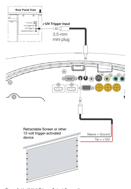
Figure 3-14. 12-Volt Trigger Output Connection
