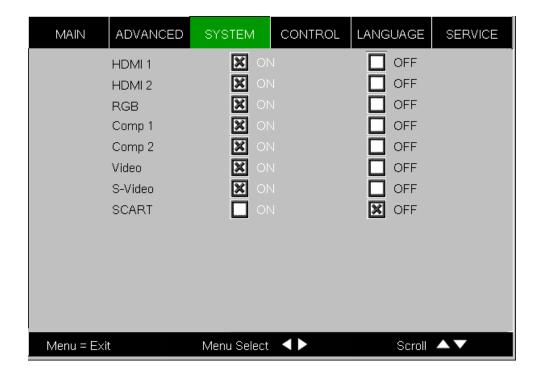
Figure 4-14. Input Enable Sub-Menu
