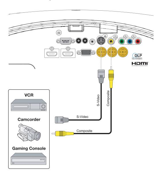
Figure 3-12. Composite and S-Video Connections
