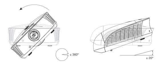
Figure 3-7. Mounting Angle Ranges (Front-to-Back and Side-to-Side)
