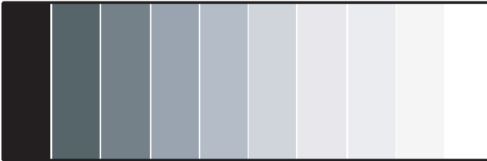
Figure 4-3. Typical Gray Bar Pattern for Adjusting Contrast
