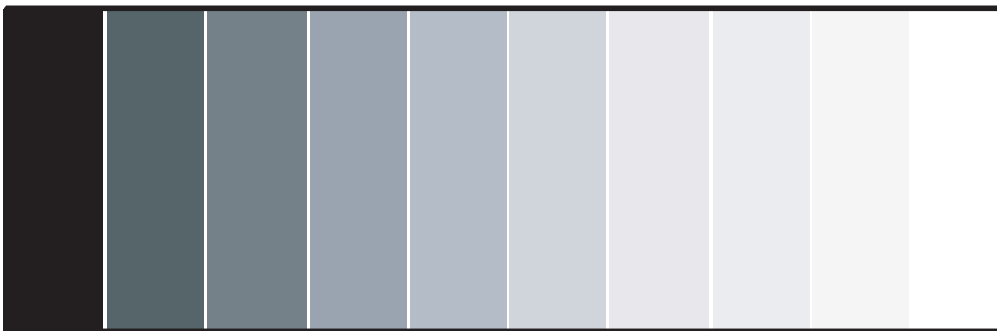
Figure 4-4. Typical Gray Bar Pattern for Adjusting Contrast
