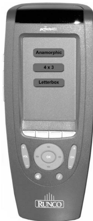
Aspect Ratio Screen: This screen will allow you to select your Aspect Ratio.
