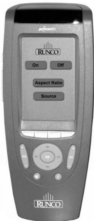
Main Screen: This screen will turn on the Projector and send you to the Aspect Ratio or Source screen.
