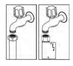
**Note:** Aquastop water spouts are used in some models. In case of using aqua stop, a dangerous tension exists. Do not cut an Aquastop water spout. Do not allow an aqua stop spout to become twisted.
