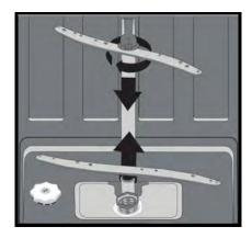
Always check the spray arm water outlet to ensure they are not clogged. If these are clogged, ensure they are cleaned.
