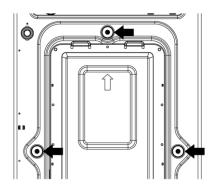
2. Unscrew the 3 screws with a 10mm hex wrench, spanner or cross-tip screwdriver. Keep the 3 screws as they will need to be re-used if the machine has to be transported.
