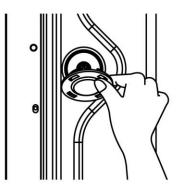
4. Adjust the level of washing machine by the adjustable feet. Please check if there is a gap between the four adjustable feet and the floor. If there is then adjust the level of the washing machine by turning the adjustable feet. Make sure that the machine does not sway and that it is completely level. After the adjustment is finished, turn the fixing nuts up tightly, so that the adjustment that has been made is fixed.
