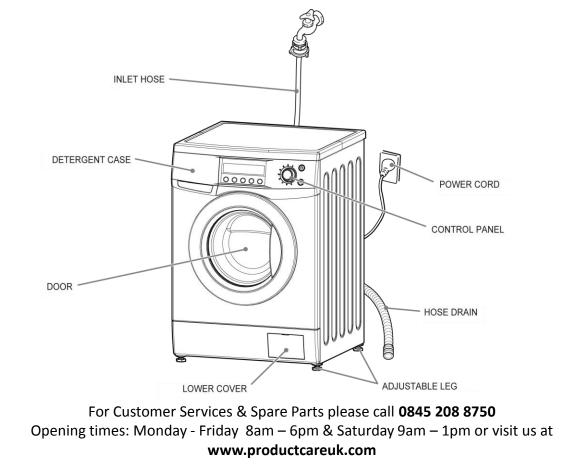
1. Before operating the washing machine, remove the 3 transportation screws and rubber spacers. If the screws are not removed, it may cause heavy vibration, noise and product malfunction, (voiding the guarantee).
