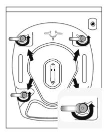
Pull out the screws together with the coloured plastic spacer, (the bolts that have been removed from the machine should be kept in case the machine needs to be used in future).
