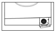
Before opening the filter cover, place a towel on the ground immediately in front of the filter hole to soak up remaining water.
