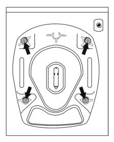
Loosen the bolts by rotating counterclockwise with a suitable spanner.
