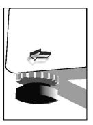
Adjust the feet upward and downward by rotating them clockwise and anticlockwise.
