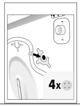
4. Adjust the level of washing machine by the adjustable feet. Please check if there is a gap between the four adjustable feet and the floor. If there is then adjust the level of the washing machine by turning the adjustable feet. Make sure that the machine does not sway and that it is completely level. After the adjustment is finished, turn the fixing nuts up tightly, so that the adjustment that has been made is fixed.
