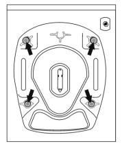
2. Unscrew the 4 screws with a wrench, spanner or cross-tip screwdriver. Keep the 3 screw as they will need to be re-used if the machine has to be transported.
