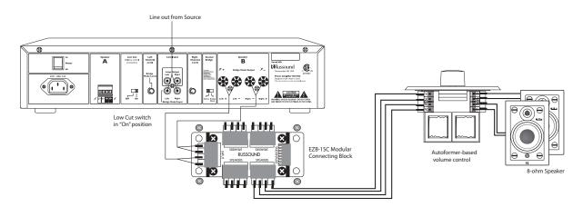
The R275HC can also be configured as a power upgrade for specific zones, for use with large speaker selectors and for long series-parallel speaker runs (e.g., outdoor zones).
