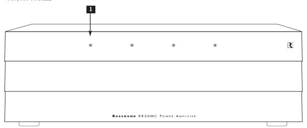
**Zone Indicator LEDs:** The four LEDs correspond to the four stereo zone amplifiers. The LED will illuminate red when the amplifier power is on and the zone is in standby. The LED will illuminate green when the zone is active.
