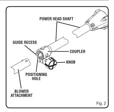
Push in the button located on the blower attachment. Align the button with the guide recess on the power head coupler and slide the two shafts together. Rotate attachment shaft until button locks into the positioning hole.
