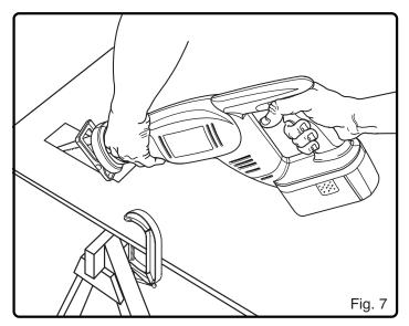
Mark the line of cut clearly. Choose a convenient starting point inside the area to be cut out and place the tip of the blade over that point. Rest front edge of base (shoe) assembly on work and hold firmly in position. Depress the lock-off button, then pull switch trigger to start the cutting action.
