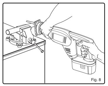
Metals such as sheet steel, pipe, steel rods, aluminum, brass, and copper may be cut with your saw. Be careful not to twist or bend the saw blade. **Do not force.** We recommend cutting oil when cutting most soft metals and steel. Cutting oil will also keep blades cool, increase cutting action, and prolong blade life.
