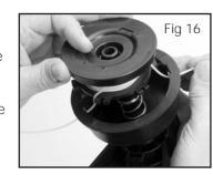
Once the spool is in place, apply pressure on the spool compressing the spring. Pull each end of the line sharply to unlock the line from the slots. Continue to apply pressure to the spool until the knob can be threaded clockwise onto
