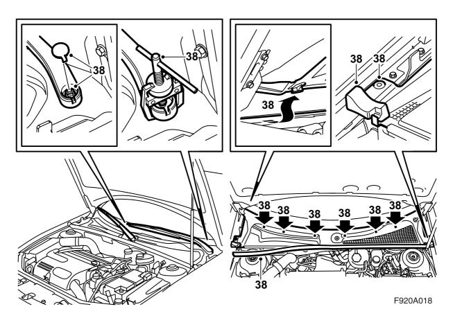
38 Remove the wiper arms using puller 85 80 144. Remove also the bonnet seal and the cover over the bulkhead space.
