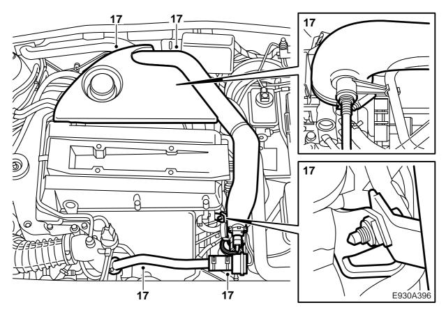
17 Remove the engine cover and disconnect any hoses and electrical connections from the turbocharger delivery pipe. Remove the turbocharger delivery pipe between the charge air cooler and the throttle body, including the bypass pipe and the heat shield over the exhaust manifold. Plug the holes.
