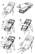
The SIM card is inserted under the phone's battery. Ensure that the phone is switched off and the charger disconnected.
