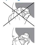
The antenna is integrated in your phone, under the back cover at the top. Avoid putting your fingers on this area when the phone is switched ON. If your fingers obstruct the antenna, the phone may have to operate with a higher power level than usual; decreasing its efficiency quickly. It could also affect the quality of your communications.
