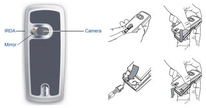
Put the strap through the hook inside and at the bottom of the phone. Pull the strap to lock it into place.
