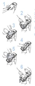
The SIM card is inserted under the phone's battery. Ensure that the phone is switched off and the charger disconnected.
