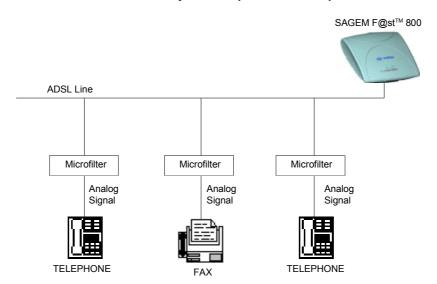
The configuration with microfilters requires one microfilter for each analog terminal.
