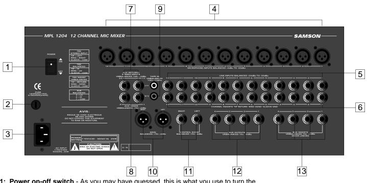
1: Power on-off switch - As you may have guessed, this is what you use to turn the MPL 1204 on and off. To avoid potential damage to your speakers, turn the MPL 1204 on *before* you turn on any connected power amps—and turn it off *after* the power amps are turned off.
