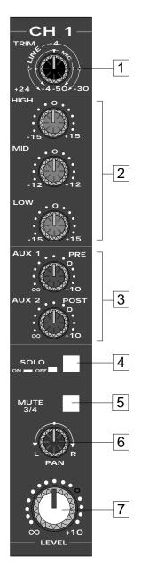
1: Trim (black) - This knob determines the input level of the connected signal. Continuously adjustable from +4 dB to -50 dB (for mic inputs) or +24 to -30 dB (for line inputs), the input signal is boosted when the trim is turned clockwise and attenuated when turned counterclockwise. For information on how to properly set this for each channel, see the section on page 14 entitled "Setting The Correct Gain Structure."
