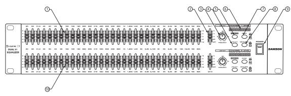
(1) Equalizer level sliders - Independent Equalizer sliders are provided for each frequency area (The S curve 231 provides 31 frequency areas). Calibration markings on either side of each Equalizer slider allow you to cut or boost each frequency area. As described below, the exact action of the Equalizer sliders depends upon the setting of the Range switch as well as the setting of the Cut Only switch (see #3 and #5).
