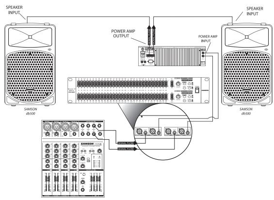
In this example the mixer's stereo output is connected to the S curve 231's inputs. Then, the S curve 231's outputs are connected to the input of a 2-channel power amp. Next, the power amplifier's outputs are connected to the passive (non-powered) loudspeakers.
