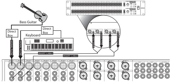
You can use the S curve 231 in your mixer's insert points if you want to equalize two mono channels individually in the mix. In this example the S curve 231's Channel 1 INPUT and OUTPUT are inserted on a bass guitar channel using a 1/4-inch TRS to  $2 \times 1/4$ -inch TS "Y" cable, and the Channel 2 INPUT and OUTPUT are inserted on a keyboard channel using the same type of cable. For more information on cable wiring see the S curve 231 Wiring Guide page 15 in this manual.
