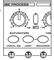
reach. Using a limiter will help you avoid unwanted peaks or overloads in the signal, which can sometime cause undesirable distortion. When the LIMIT switch is pressed in, the yellow LED will illuminate indicating the C Valve is limiting the signal.
