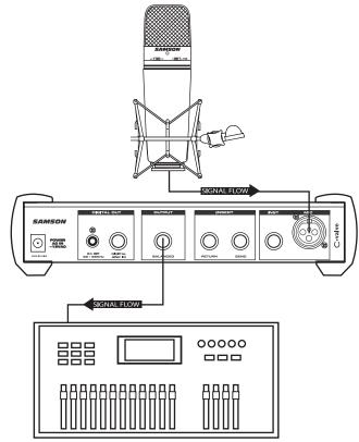
At this point you should be sending a clean signal to your mixer or recorder and you can experiment with the SATURATION, VOCAL EQ and ENHANCER features for fun. A detailed explanation of these functions will be covered in the following sections of this manual.
