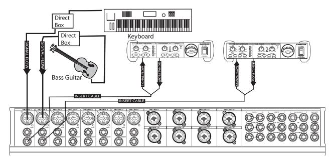
You can use the C valve to "warm-up" the signal from recorded tracks or instruments such as digital electric piano or bass, to name a couple. The example above shows the two C valves inserted into the insert point of a mixer on the keyboard and bass channels. Set the input and output level so that you get unity gain (the same level in and out), and then use the SATURATION control to adjust the amount of tube sound.
