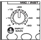
+6dB. If you see the OL LED light you are "Over-Loading" and the sound may become distorted. If this happens, simply back down on the INPUT GAIN control until the OL light stops flashing.
