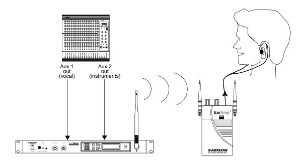
Similarly, if you're a guitarist, you can route guitar signal only to one mixer aux send and a mix of all other signals to the other mixer aux send; the Wireless EarAmp® Balance control will then give you the ability to hear as much or as little of your instrument—relative to the overall mix—as you like.
