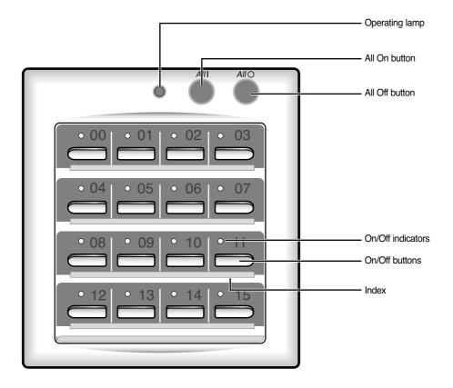
More Operating lamp comes on when at least one air conditioner connected to the centralized controller is operating.
