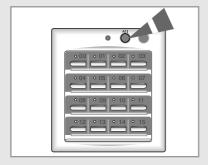
Up to sixteen air conditioners can be turned on or off by connecting to the centralized controller. However, you cannot adjust the cooling temperature or set the timer with it. If you also have the wired remote controller, CENTRALIZED CONTROL is displayed at the top of the remote controller.
