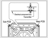
3 Secure the transmitter with four spacer supports into the electrical component box.
