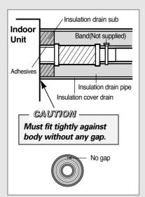
Care must be taken when installing the drain hose for the indoor unit to ensure that any condensate water is correctly drained outside.
