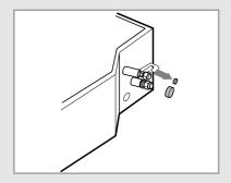
On delivery, the indoor unit is loaded with an inert nitrogen gas. All this gas must therefore be purged before connecting the assembly piping. To purge the inert gas, proceed as follows.
