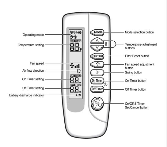
Mote After cleaning the air filter, press the filter reset button.
