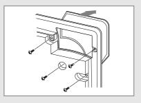
In case of using the wireless remote controller, you must install the receiver & display unit to the front panel before fixing the panel.
