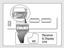
4 Connect the end of the connector wire to the receiver & display unit and connect the other end of the wire to the electrical component box as shown in figure.
