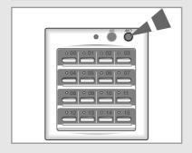
3 To turn off the all of air conditioners connected to the centralized controller, press the  $\bigcap^{\text{MO}}$  (All OFF) button.
