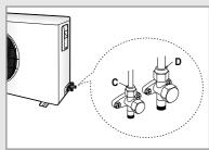
Before completing the installation (insulation of the hose and piping), you must check that there are no gas leaks.
