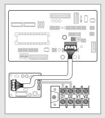
4 Connect the cable from the PCB to the transmitter. And connect another cable from the O1, O2 terminals to the transmitter as shown in figure.
