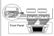
2 Connect the cables of the front panel to the PCB as shown in figure.
