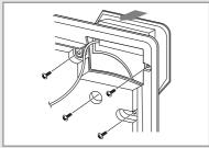
3 Secure the receiver & display unit with the screws, then install the insulation.
