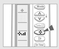
3 Select the fan speed by pressing the button one or more times until the required setting is displayed:
