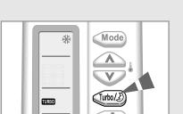
The Turbo cooling/heating function is used to cool or heat your room as quickly as possible.
