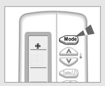
2 If the is not displayed at the top of the remote control, press the button on the remote control one or more times until it appears.
