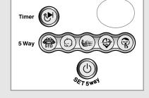
2 To stop the operating, press the (I) (On/Off) button until all indicators turn off.
