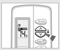
3 To adjust the temperature, press the TEMPERATURE buttons one or more times until the required temperature is displayed. Possible temperatures are between 65°F(18°C) and 86°F(30°C) inclusive.
