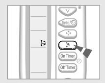
Depending on the position of the indoor unit on the wall of your room, you can adjust the position of the outer air flow blade on the bottom of the unit, thus increasing the efficiency of the air conditioner.
