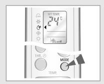
2 Press the button on the remote control until 𝒇◀ is displayed.
