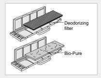
The air conditioner can be fitted with a deodorizing and Bio-Pure filter to remove minute dust particles or odours. The service life of the filter is approximately three months depending on the time during which the air conditioner is used.
