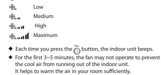
Note: Silence mode(%) makes the noise quieter during operating the indoor unit in the Heat mode.
