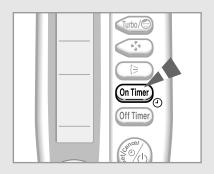
The On Timer enables you to switch on the air conditioner automatically after a given period of time. You can set the period of time from 30 minutes to 24 hours.
