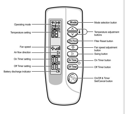
*Note* After cleaning the air filter, press the filter reset button.
