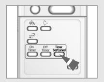
The On Timer enables you to switch on the air conditioner automatically after a given period of time. You can set the period of time from 30 minutes to 24 hours.
