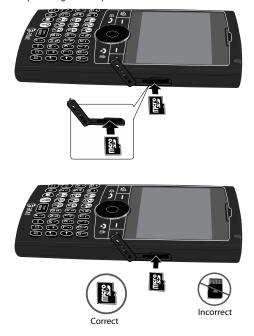
Warning!: The following illustration is the incorrect method for inserting the microSD card. If attempted, damage to the accessory port occurs therefore voiding the phone's warranty.
