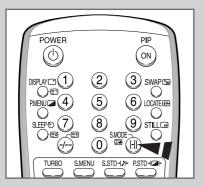
The "S.MODE" button displays/controls the processing and output of the audio signal. When power is switched ON, the mode is automatically preset to either "Dual-I" or "Stereo", depending on the current transmission.
