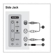
Please be sure to match the color coded input terminals and cable jacks. When both the side and rear jacks (AV IN 2) are connected to external equipment, the side receives priority.
