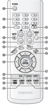
POWER Used to switch the TV on and off.
